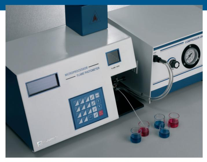
The PG Instruments FP902 Flame Photometer offers the combination of clinical, industrial and education applications in ONE instrument. It gives accurate, fast and precise analysis of sodium, potassium, calcium and lithium in one simple aspiration.
